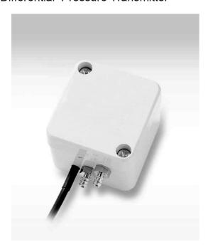
EQD model is ideal for the application (such as HVAC) with differential pressure, vacuum pressure, gauge pressure and especially low pressure of non-corrosive gases or air measured. Analog output 4~20mA, 2wire.
