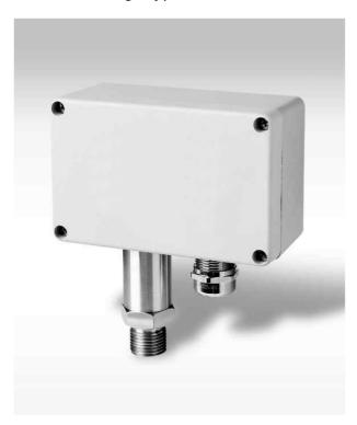
QCN model is high precise and its media-wetted materials are composed of stainless steel 316, having excellent corrosion-resistant properties. It is applied to precise measurement and builds an amplifier therein to interface with various kinds of controllers. Wall Mounting type which is easy to attach on wall.
