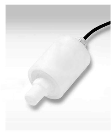
QDB, QDE designed for high precision measurement and consist of ceramic pressure cell. QDB made of QUGF or QUB, the material of component can be against corrosion, it has no seal inner part. QDE precision pressure cell is surrounded by TEFLON and corrosion-resisting O-ring is airtight. These specification be good at corrosion proof, QDE applies to various control equipment.
