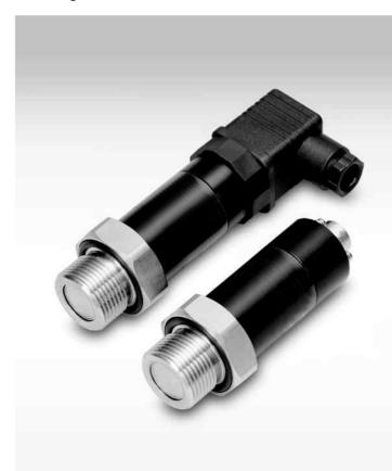
QTI(Flush Diaphragm) model is designed as a flush diaphragm suitable for sanitary use and is high precise for tank levels. Media-wetted materials there are composed by stainless steel 316L to have superior corrosion-resistant properties. It is applied to precise measurement and builds an inner amplifier to interface with various kinds of controllers.
