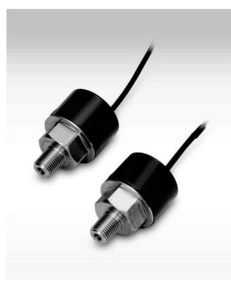
QTP sensing element has excellent temperature properties by adopting a self temperature compensation foil strain gauge. A diaphragm and a pressure port are composed as one body for the prevention of leakage. It is also durable to an instant over pressure. It can control the system without any controller due to the output of a 1 or 2 channel NPN open collector switch.
