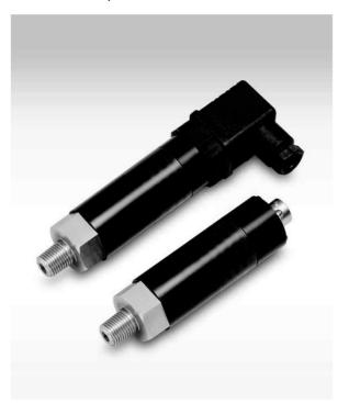
QUB model has applied Silicon Piezoresistive cell, which attached High Temperature Glass on Titanium. Since it does not use O-ring, there is no possibility of corrosion and leak. Its low price makes it suitable for industrial uses. With its various outputs, it may be interfaced with various controllers.
